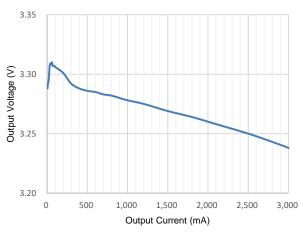
Figure 9. Load Regulation, Vout=3.3V
