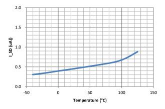
Figure 3. Shut-down Current vs Temperature
