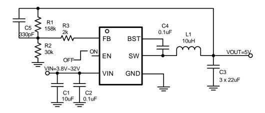
Figure 15. 24V Input, 5V/3A Output
