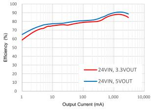
Figure 1. Efficiency vs Load Current, Vin=24V
