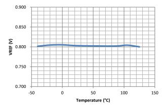
Figure 5. Reference Voltage vs Temperature
