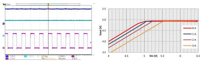
Figure 13. SCT2330 Switching Node Waveform
