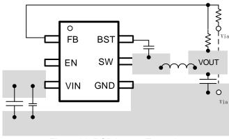
Figure 22. PCB Layout Example
