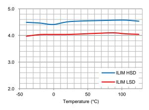
Figure 6.Peak Current Limit vs Temperature
