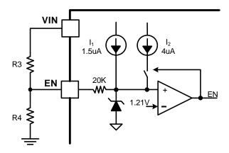
Figure 12. Adjustable VIN UVLO
